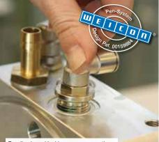
Bonding in and locking screw connections of a pressure unit
