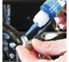
Bonding a stainless-steel screw into a housing
